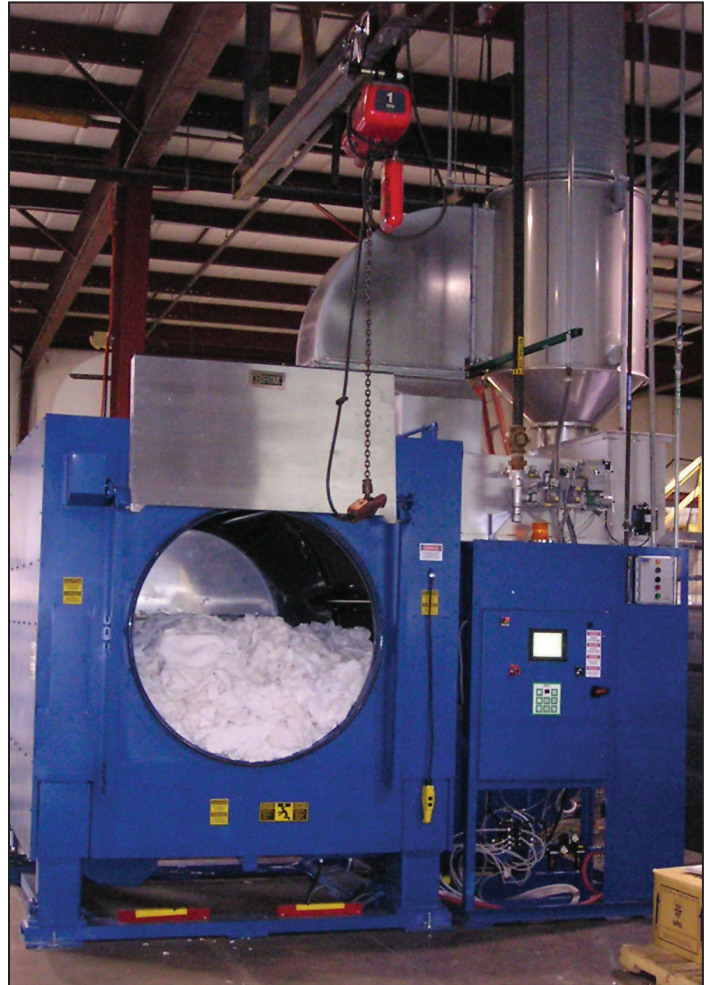
This lint filter is shown in a one-on-one, or inline, application with a dryer.
